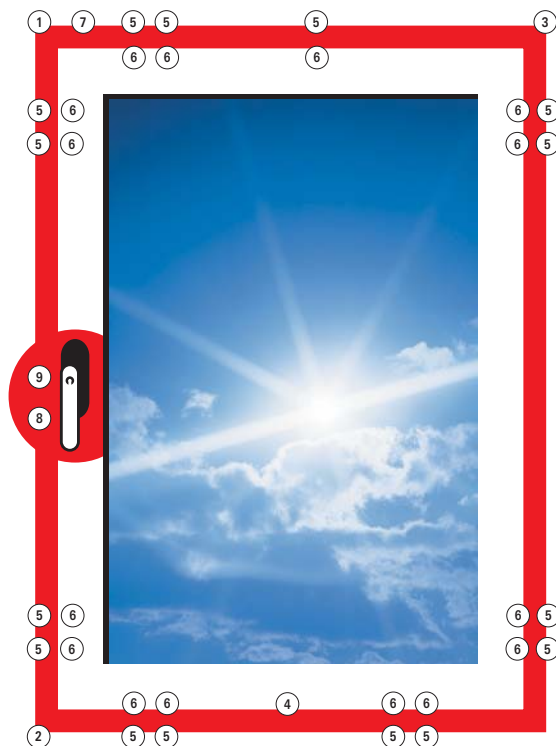
In RC3 windows all corners are secured twice
