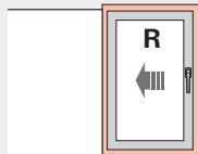
Diagram B 1 sliding sash (L or R) Inside frame flush with the wall
